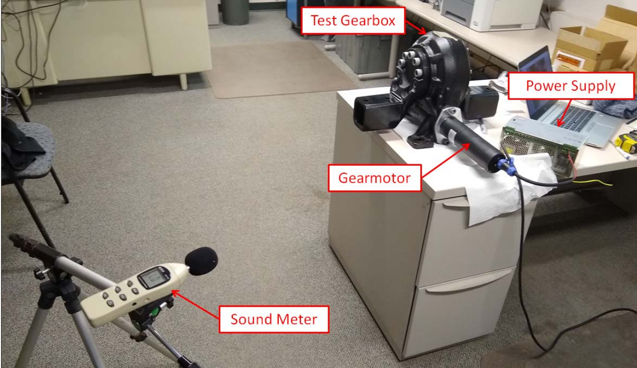
Figure 4. Dynamic Test Setup in Control Room
