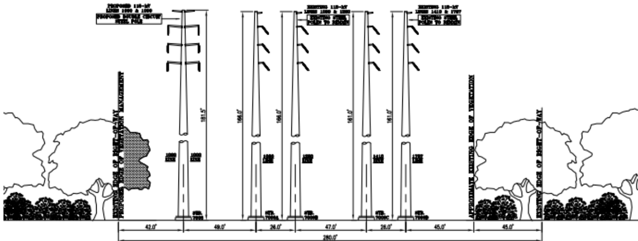
PROPOSED R.O.W. CONFIGURATION DOUBLE CIRCUIT STEEL MONOPOLE DESIGN LOOKING FROM MONTVILLE SUBSTATION TO NORTH OF KITEMAUG ROAD IN THE TOWN OF MONTVILLE, CT STR. #7608
