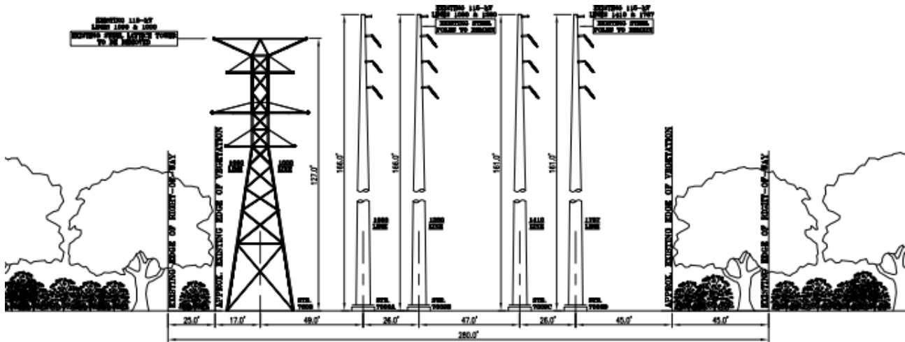
EXISTING R.O.W. CONFIGURATION DOUBLE CIRCUIT STEEL LATTICE TOWER DESIGN LOOKING FROM MONTVILLE SUBSTATION TO NORTH OF KITEMAUG ROAD IN THE TOWN OF MONTVILLE, CT STR. #7608
