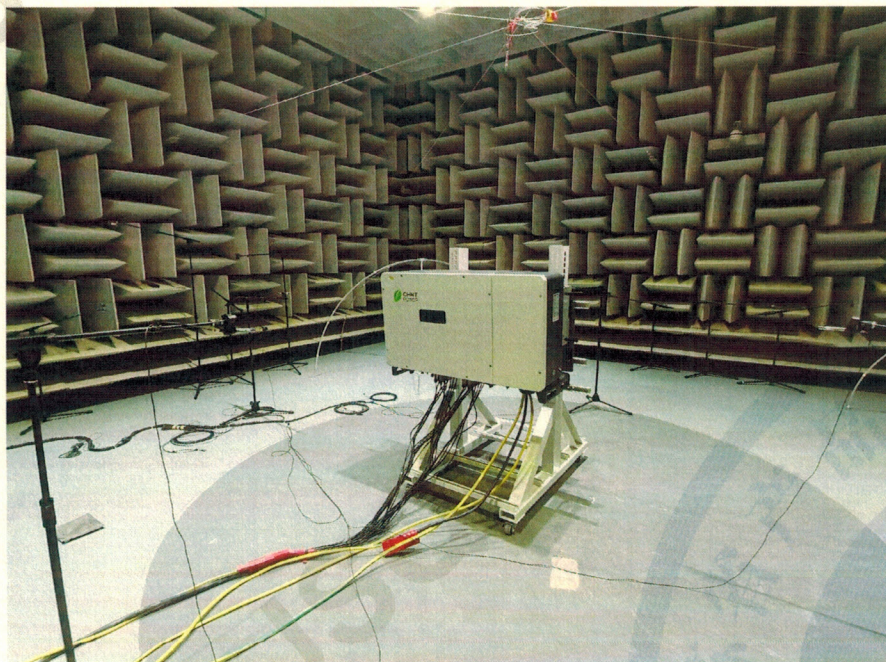
Figure 1 – Measurement surface – parallelepiped – with key microphone positions
