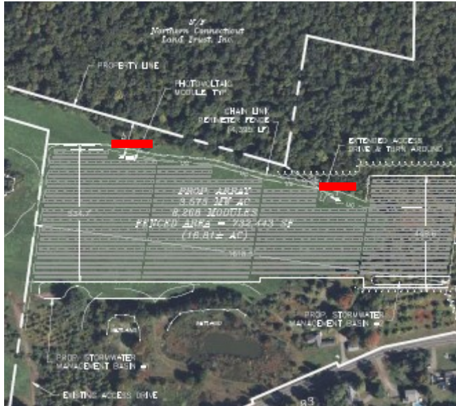
Figure 5. Recommended Location for the Noise Barriers
