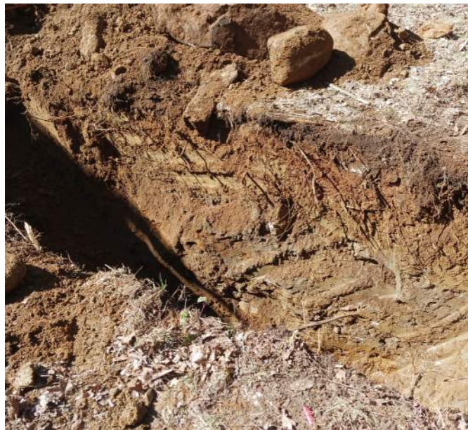
Bottom of test pit at 7.5 feet. Picture showing soil strata at Test Pit 6
