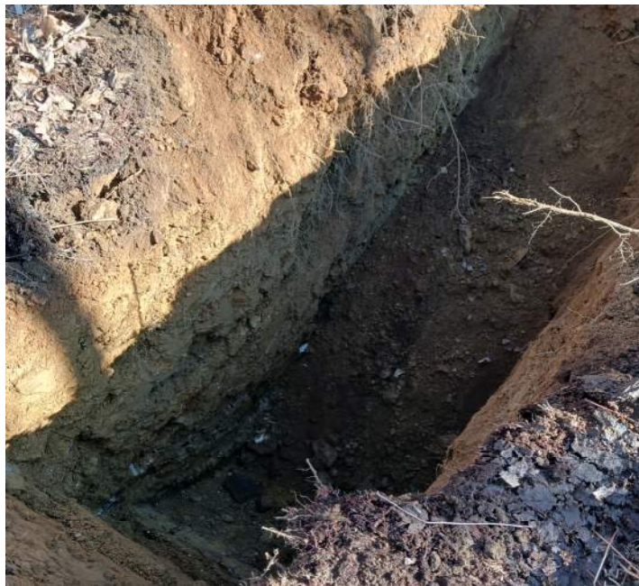
Bottom of test pit at 7.5 feet. Picture showing soil strata at Test Pit 1
