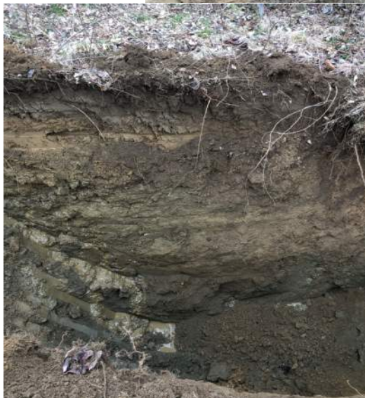
Bottom of test pit at 8.3 feet. Pictures showing soil strata at Test Pit 5.
