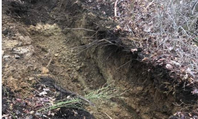
Bottom of test pit at 7.8 feet. Pictures showing soil strata at Test Pit 6
