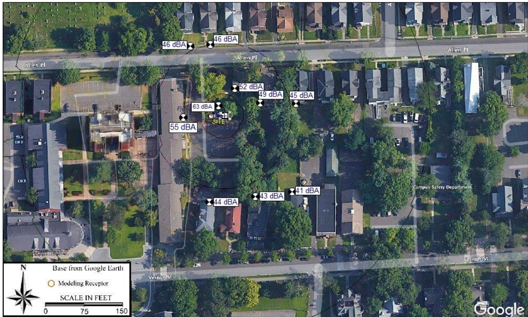
Figure 3: Graphical Summary of Predicted SOFC Sound Levels with a modest Liner on the East End
