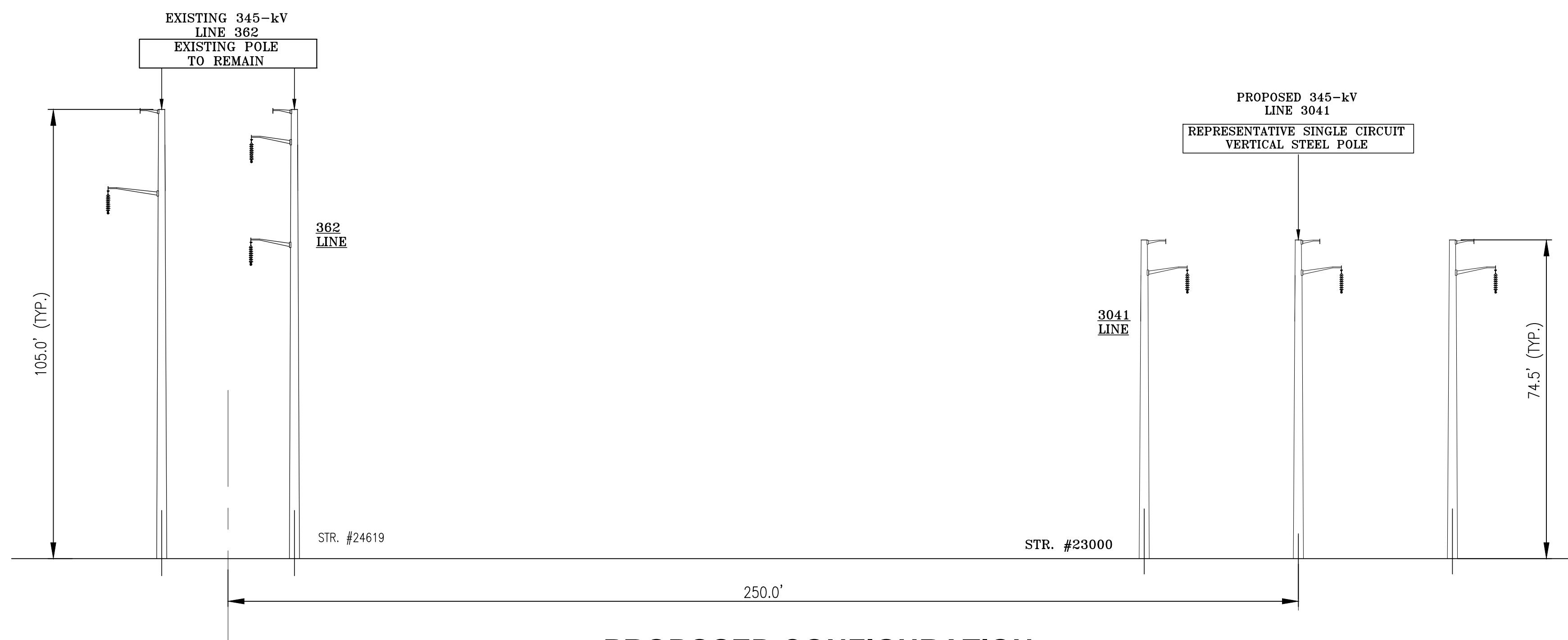
PROPOSED CONFIGURATION NO ADDITIONAL RIGHT-OF-WAY REQUIRED SINGLE CIRCUIT THREE POLE DESIGN LOOKING WEST FROM SCOVILLE ROCK SUBSTATION TO CHESTNUT JUNCTION IN THE CITY OF MIDDLETOWN, CT STR. #23000
