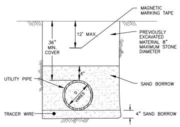
NOTES: 1 COMPACT ALL BACKFILL MATERIAL WITH VIBRATORY PLATE EQUIPMENT (MINIMUM TWO PASSES) TO A MINIMUM DENSITY OF 95 PERCENT OF THE STANDARD PROCTOR DENSITY AS
