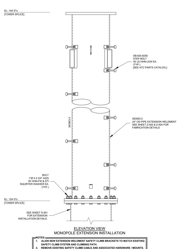
INSTALL NEW ATC-APPROVED SAFETY CLIMB SYSTEM WITH NEW 3/8"Ø SAFETY CLIMB CABLE. ENSURE 100% TIE-OFF IS MAINTAINED AND CABLE IS FREE OF ALL
