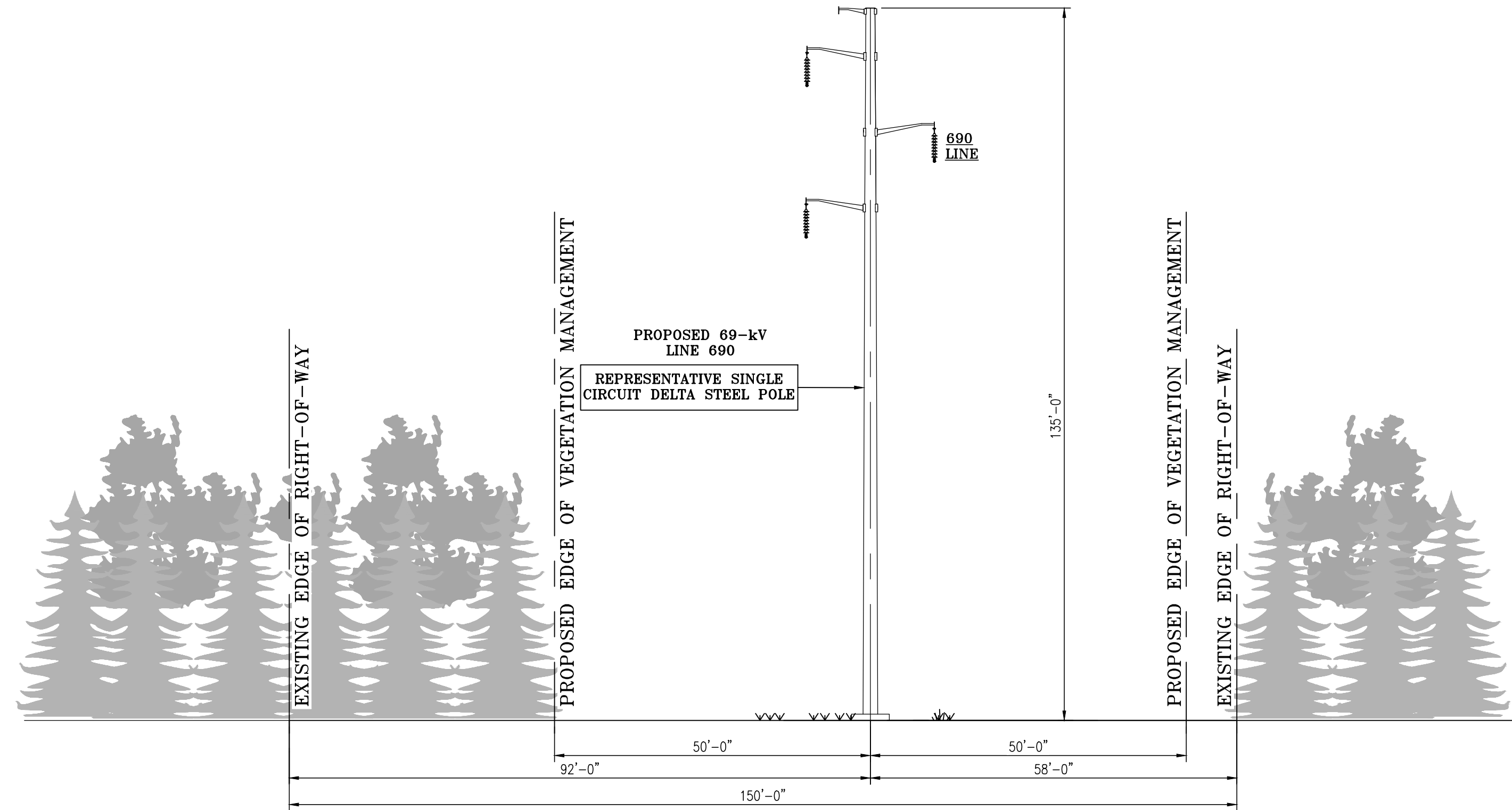
PROPOSED R.O.W. CONFIGURATION NO ADDITIONAL RIGHT-OF-WAY REQUIRED SINGLE CIRCUIT STEEL POLE DELTA DESIGN LOOKING FROM SALISBURY SUBSTATION TO NY/CT BORDER IN THE TOWN OF SHARON, CT STR. #1062
