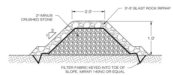
. STONE SHALL BE PLACED MECHANICALLY OR BY HAND. STONE SHALL NOT BE DUMPED DIRECTLY INTO SWALE. 2. SEE GRADING AND DRAINAGE PLAN.
