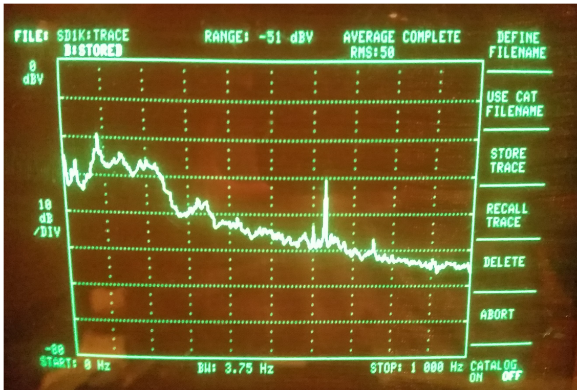
Figure 7. Discrete Tones Produced by Fuel Cell Cooling Module (0 dBV = 88.6 dB re20 \mu Pa)
