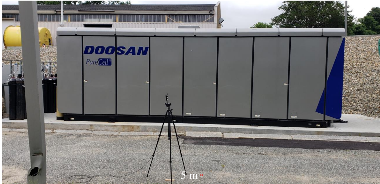
Figure 6. Sensor at 5-Meters (South) from the Power Module at the Montville Site
