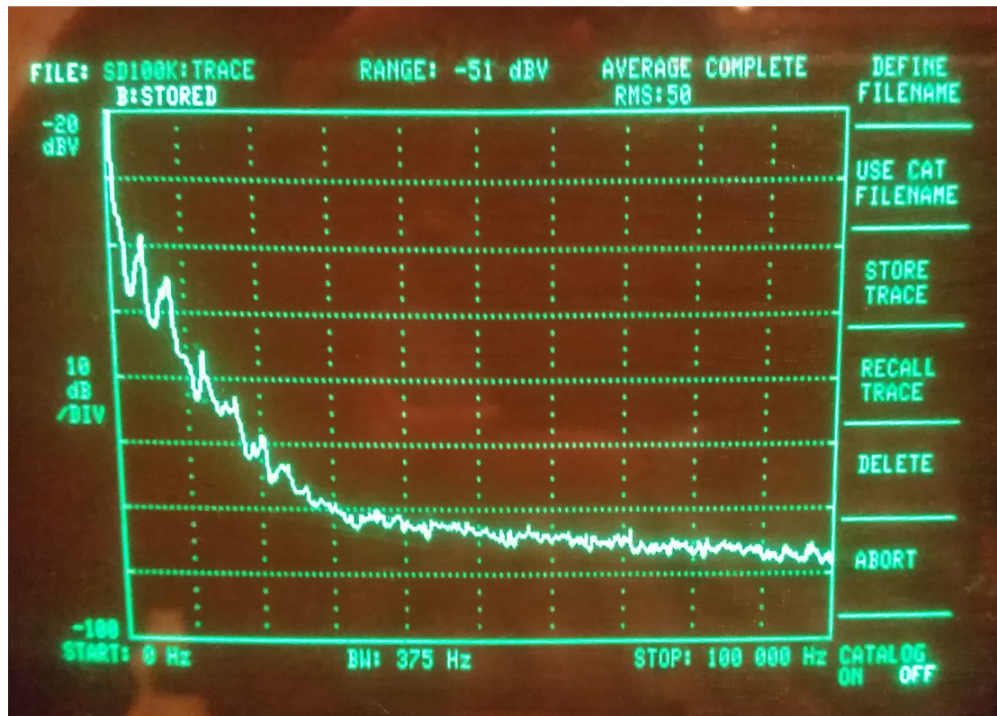
Figure 9. Ultrasonic Noise from the Fuel Cell Cooling Module (0 dBV = 88.6 dB re 20μPa)
