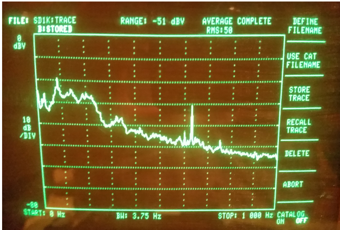
Figure 8. Infrasonic Noise from the Fuel Cell Cooling Module (0 dBV = 88.6 dB re 20 \mu Pa)
