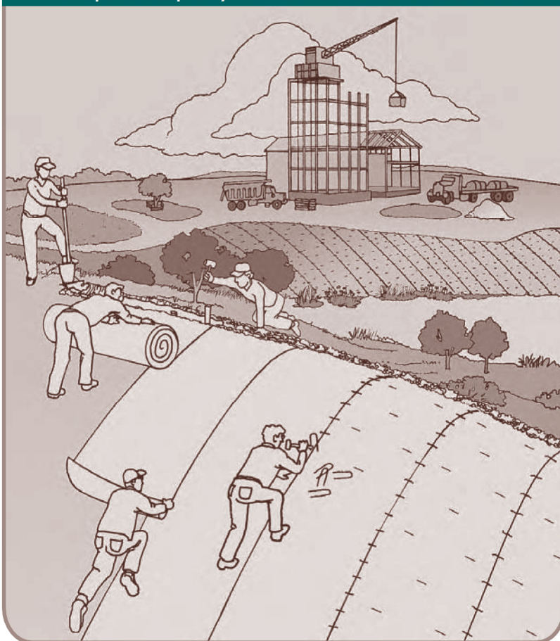
Figure ECB-1 Example of Temporary Erosion Control Blanket Installation
