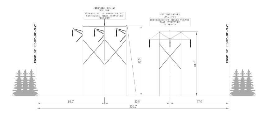
PROPOSED R.O.W. CONFIGURATION NO ADDITIONAL RIGHT-OF-WAY REQUIRED LOOKING FROM SOUTHINGTON SUBSTATION TO BLACK POND JUNCTION STRUCTURE #9550
