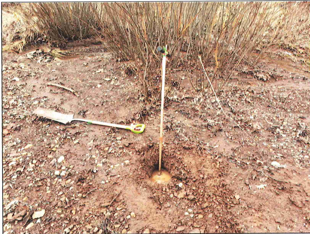
Photo 2: Exploratory soil pit, southern portion of "pond"; facing southerly
