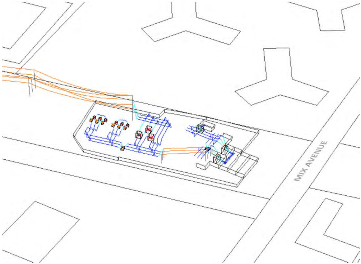
Figure 7. Overview of the three-dimensional SUBCALC model used to calculate magnetic fields for the proposed configuration of the Mix Avenue Substation.
