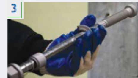
3 Move the collapsible washer to the correct location on the tool and fold in place.
