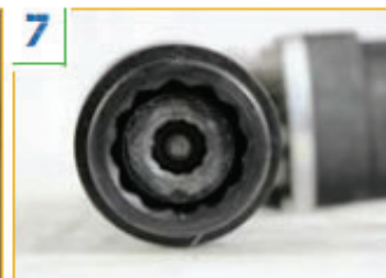
7 Using the shear wrench engage the outer socket with the splined end of the bolt. Press the trigger until correct tension has been achieved (the bolt spline separates from the bolt).
