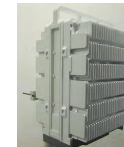
ERICSSON RADIO 4449 B71+B85 DIMENSIONS: 14.9"H x 13.2"W x 9.3"D WEIGHT: 74.0 lbs QUANTITY: 1 PER SECTOR, TOTAL OF 3
