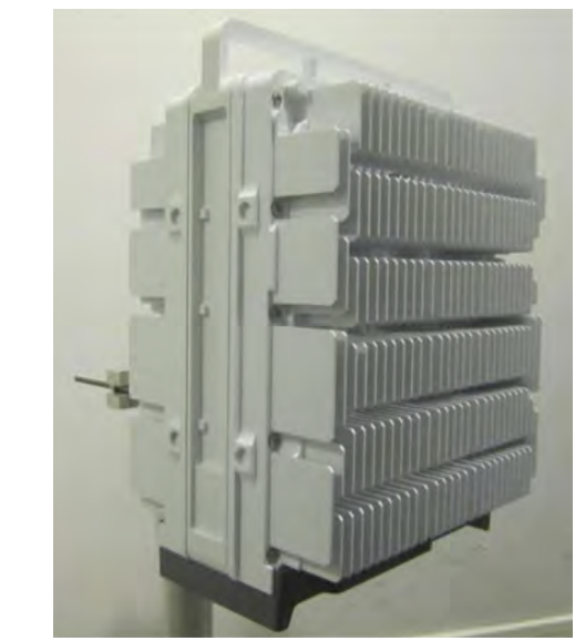
ERICSSON RADIO 4449 B71+B85 DIMENSIONS: 14.9"H x 13.2"W x 9.3"D WEIGHT: 74.0 lbs QUANTITY: 1 PER SECTOR, TOTAL OF 3
