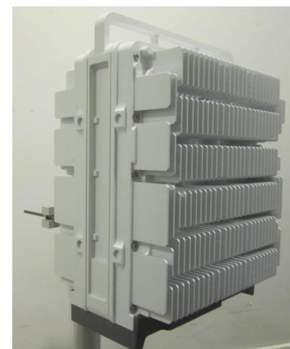
ERICSSON RADIO 4449 B12+B71 DIMENSIONS: 14.9"H x 13.2"W x 9.3"D WEIGHT: 74.0 LBS 1 PER SECTOR, TOTAL OF 3
