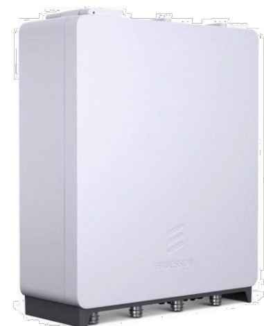
ALPHA, BETA, & GAMMA SECTORS ERICSSON RRUS 4415 B25 DIMENSIONS: 16.5"H x 13.4"W x 5.9"D WEIGHT: 46 LBS 1 PER SECTOR, TOTAL OF 3
