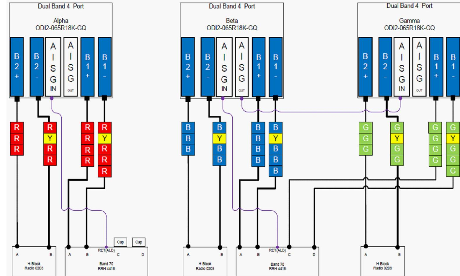
Note: This Plumbing Diagram does not represent the position of the RRUs or Antennas on the mount. That is stipulated in the Construction Drawings. If there is any question please address your Construction Manager before proceeding.
