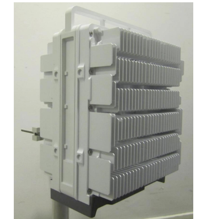
ERICSSON RADIO 4449 B12+B71 DIMENSIONS: 14.9"H x 13.2"W x 9.3"D WEIGHT: 74.0 LBS 1 PER SECTOR, TOTAL OF 3
