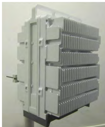
ERICSSON RADIO 4449 B71+B85 DIMENSIONS: 17.9"H x 13.1"W x 10.6"D WEIGHT: 75.0 lbs QUANTITY: 1 PER SECTOR, TOTAL OF 3
