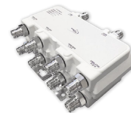
MICRODATA MI-54844 QUAD (8:4) B66/B25+B41 DIPLEXER DIMENSIONS: 4.3"H x 9.4"W x 3.5"D WEIGHT: 11.0 lbs QUANTITY: TOTAL OF 3
