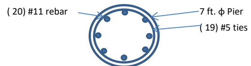
Monopole Pier Foundation
