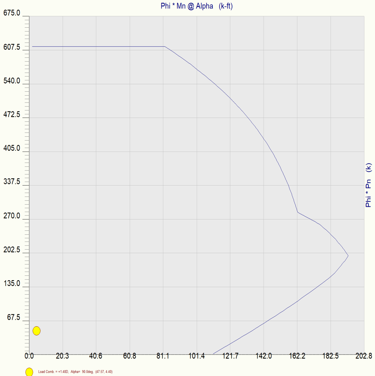
Concrete Column P-M Interaction Diagram
