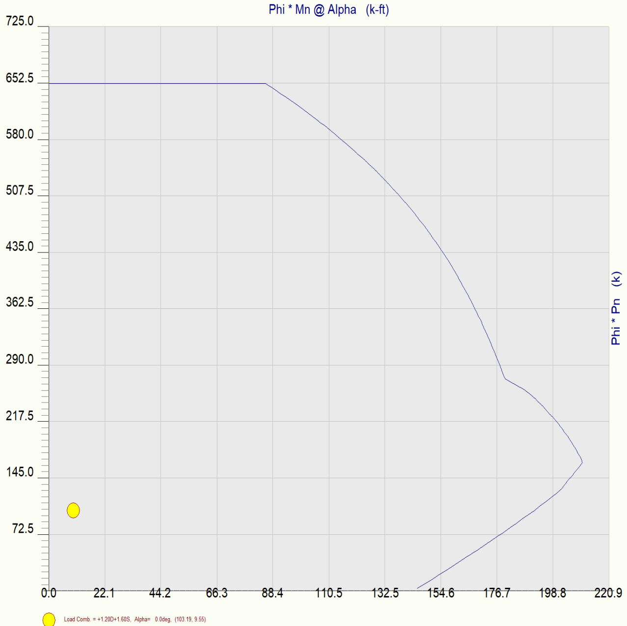
Concrete Column P-M Interaction Diagram
