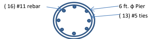
Monopole Pier Foundation
