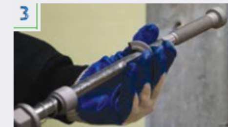
Move the collapsible washer to the correct location on the tool and fold in place.
