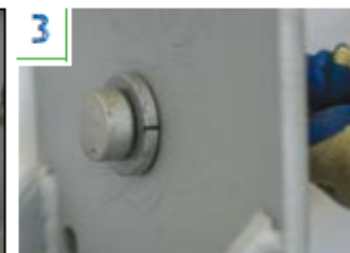
Pulling back, rock the tool side-to-side to engage the collapsible washer.
