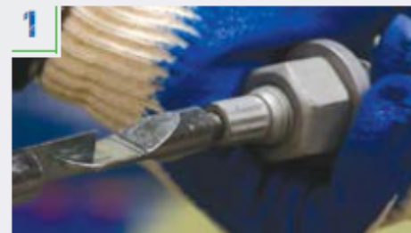
Thread the installation tool tip into the splined end of the bolt.
