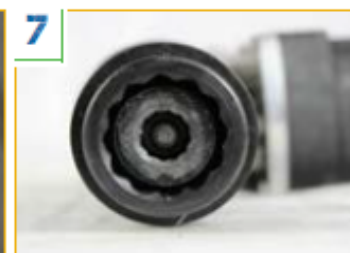
Using the shear wrench engage the outer socket with the splined end of the bolt. Press the trigger until correct tension has been achieved (the bolt spline separates from the bolt).
