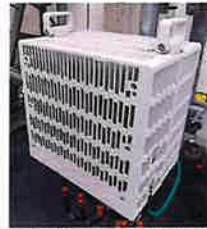
SAMSUNG RF4439d-25A B2/B66A RADIO DIMENSIONS: 15.0"H x 15.0"W x 10.0"D WEIGHT: 74.7 lbs QUANTITY: 1 PER SECTOR, TOTAL OF 3 SECTORS: ALPHA, BETA, GAMMA
