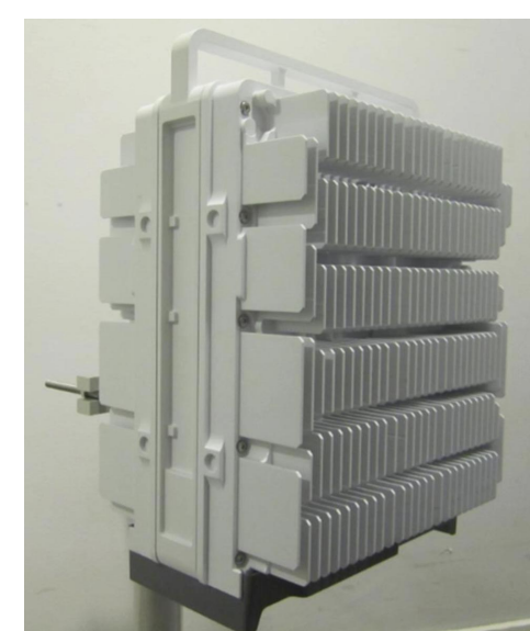
ERICSSON RADIO 4449 B12+B71 DIMENSIONS: 14.9"H x 13.2"W x 9.3"D WEIGHT: 74.0 LBS 1 PER SECTOR, TOTAL OF 3
