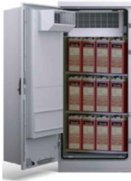
ERICSSON B160 BATTERY CABINET ENCLOSURE: ALUMINUM DIMENSIONS (HxWxD): 63" X 26" X 26" WEIGHT: 188LBS (EXCLUDES EQUIPMENT) WEATHER TIGHTNESS: NEMA TYPE 3R
