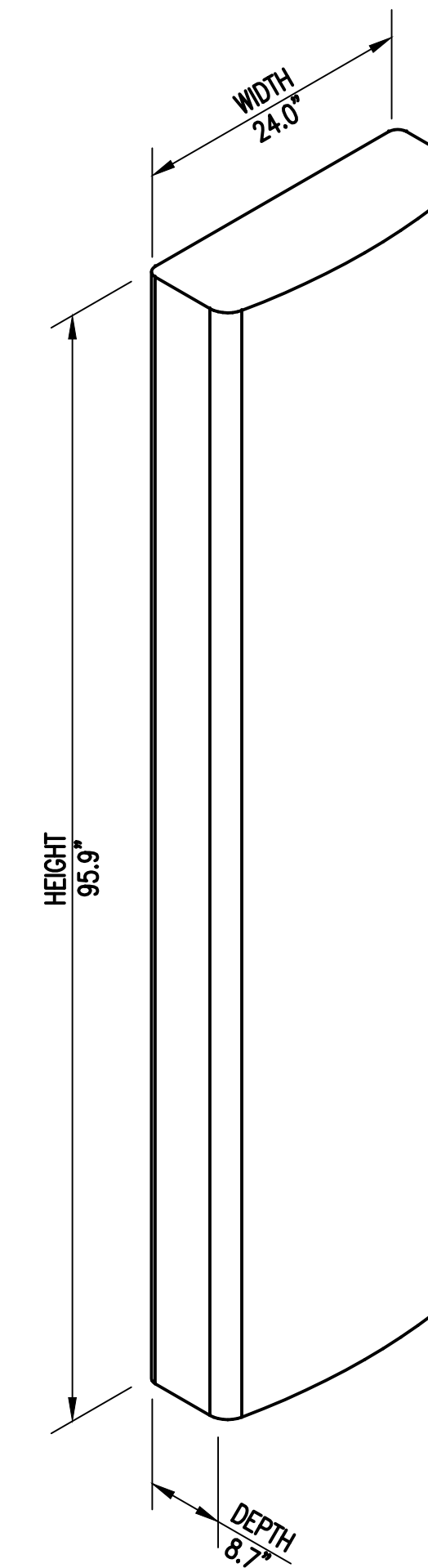
RFS APXVAARR24_43-U-NA20 PANEL ANTENNA DIMENSIONS: 95.9"H x 24.0"W x 8.7"D WEIGHT: 128.0 LBS 1 PER SECTOR, TOTAL OF 3
