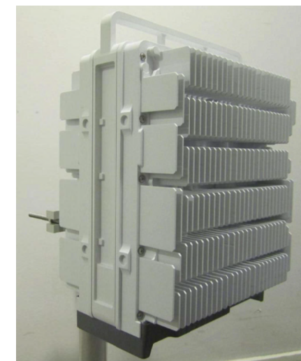
ERICSSON RADIO 4449 B71+B85 DIMENSIONS: 14.9"H x 13.2"W x 9.3"D WEIGHT: 74.0 lbs QUANTITY: 1 PER SECTOR, TOTAL OF 3
