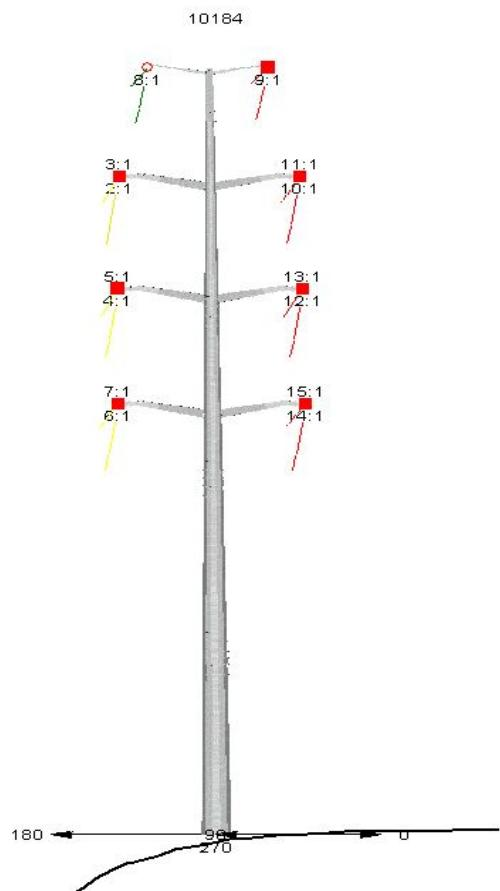
Looking south. OPGW attached on top left arm. Alumoweld attached on top right arm.
