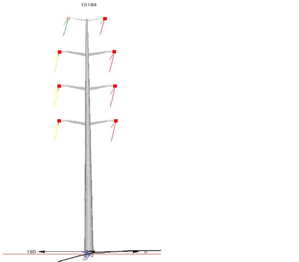
Looking south. OPGW attached on top left arm. Alumoweld attached on top right arm.
