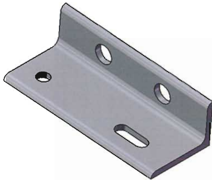
CP-00685-01 SAFETY CLIMB BASE TERMINATION ANGLE QTY: 1 WEIGHT: 2.4 LBS
