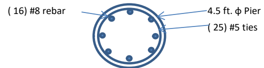
Monopole Pier Foundation
