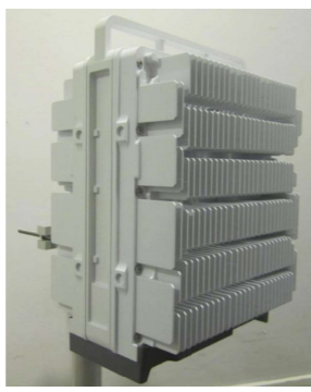
ERICSSON RADIO 4449 B12+B71 DIMENSIONS: 14.9"H x 13.2"W x 9.3"D WEIGHT: 74.0 LBS 1 PER SECTOR, TOTAL OF 3
