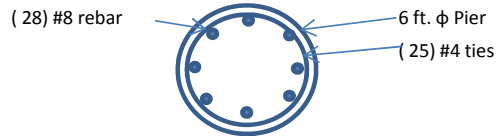
Monopole Pier Foundation
