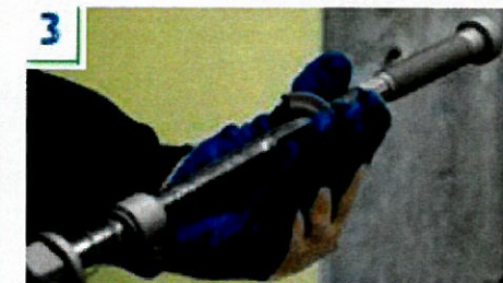
3 Move the collapsible washer to the correct location on the tool and fold in place.
