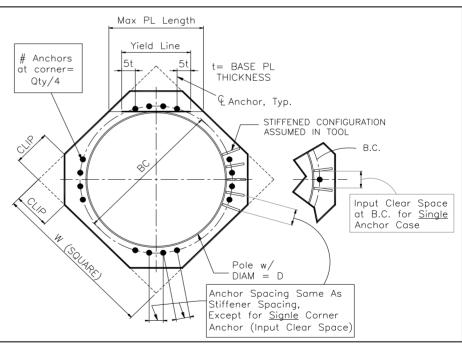
\*\* Note: for complete joint penetration groove welds the groove depth must be exactly 1/2 the stiffener thickness for calculation purposes
