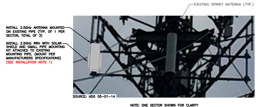
2.5 ANTENNA AND RRH PHOTO DETAIL AND EQUIPMENT SCHEMATIC SCALE: N.T.S.
