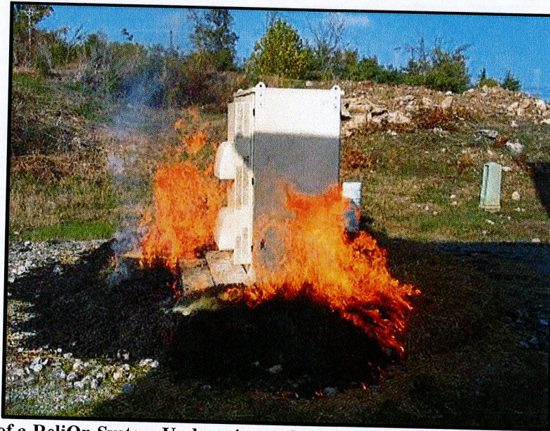
Actual Photo of a ReliOn System Undergoing and Passing the NEBS Standards Brushfire Test
