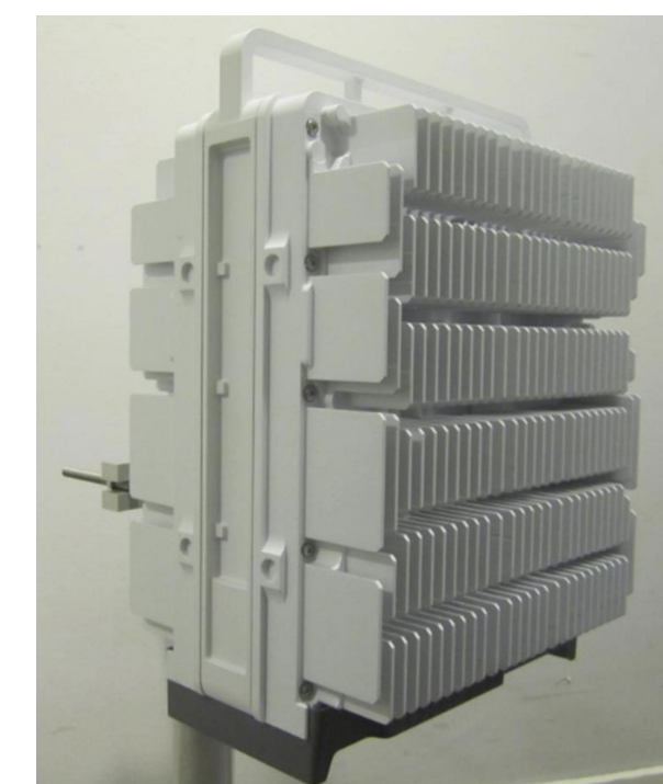
ERICSSON RADIO 4449 B12+B71 DIMENSIONS: 14.9"H x 13.2"W x 9.3"D WEIGHT: 74.0 LBS 1 PER SECTOR, TOTAL OF 2
