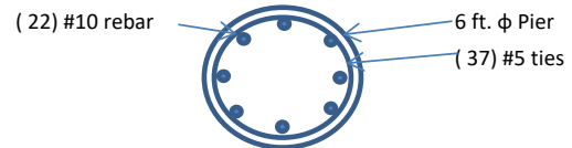
Monopole Pier Foundation
