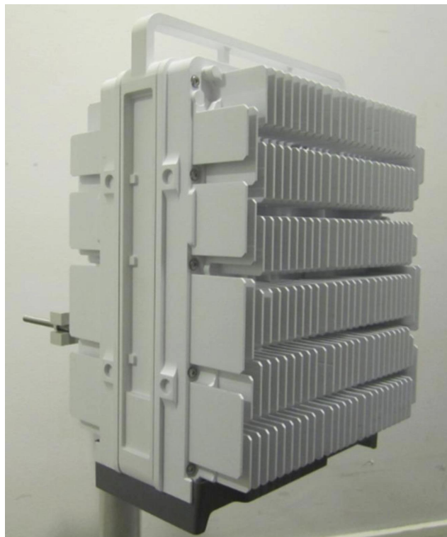
ERICSSON RADIO 4449 B12+B71 DIMENSIONS: 14.9"H x 13.2"W x 9.3"D WEIGHT: 74.0 LBS 1 PER SECTOR, TOTAL OF 3 RRU DETAIL SCALE: N.T.S.
